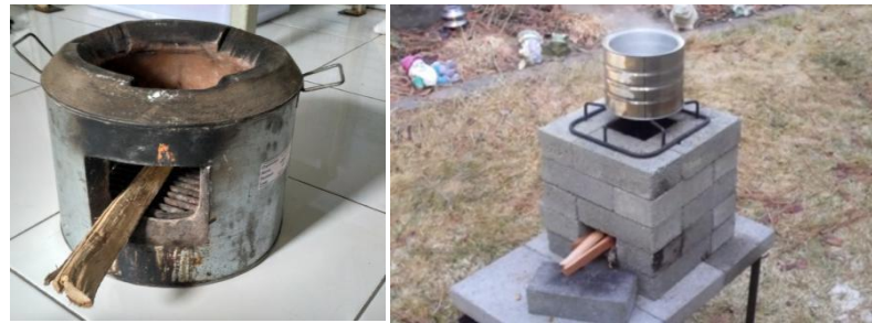
Figure 1. Keren Stove and Rocket Stove
