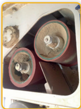
Figure 3: Rubber roller huskers
