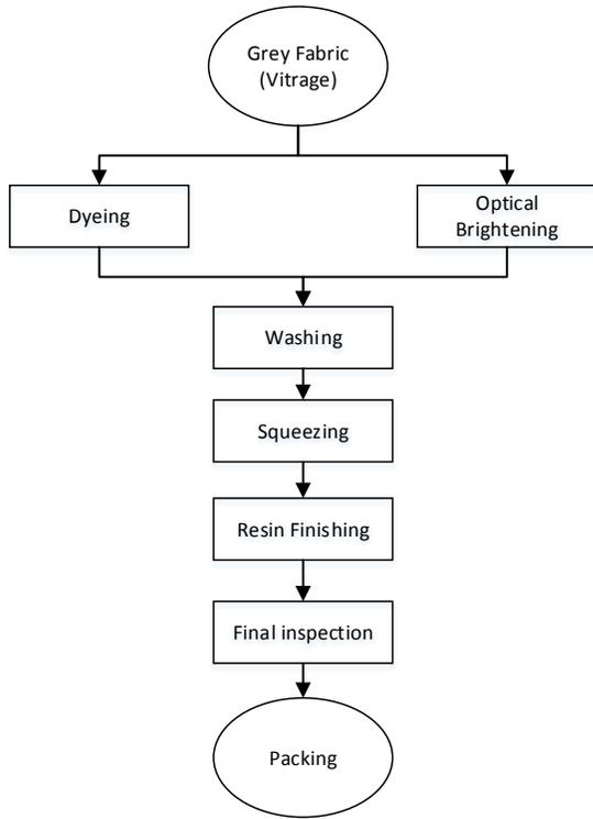
Flow process diagram for Polyester vitrage fabric
